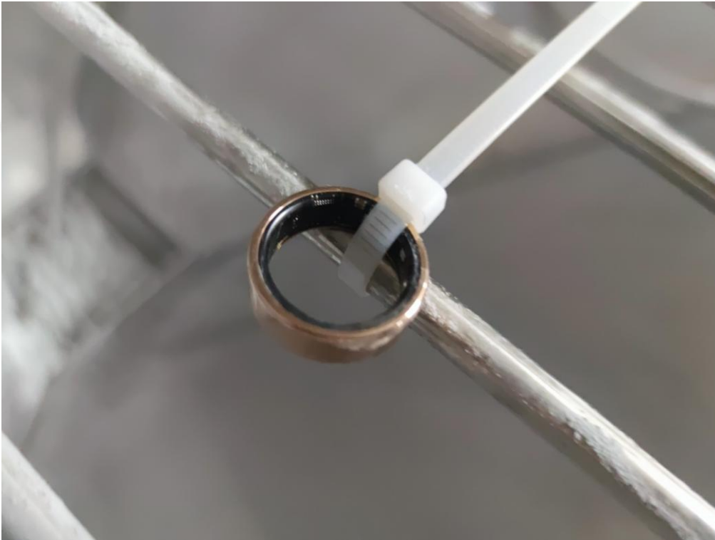
Photo 5 Before test view (IP6X)
